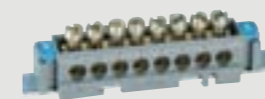
^ Unprotected terminal blocks on supports are generally fixed on 12 x 2 flat bars for connecting protective conductors
